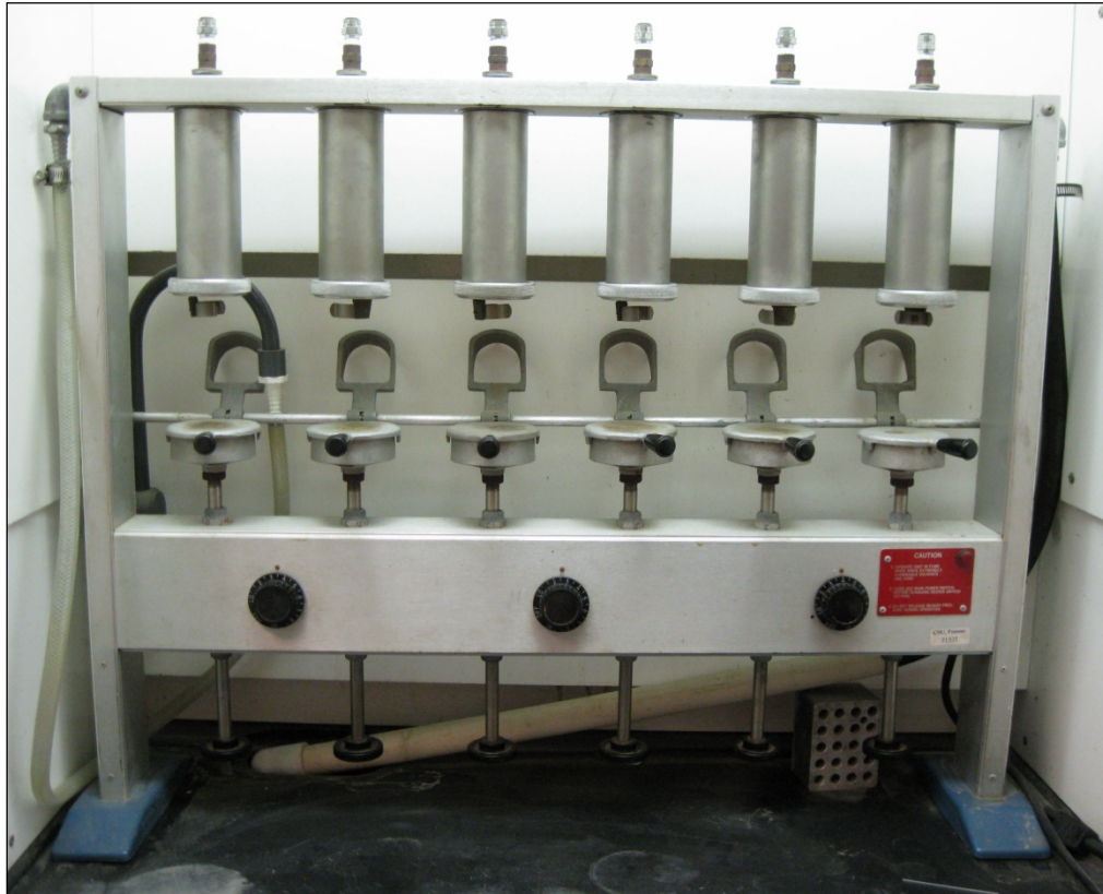
Figure 6 – Goldfish fat extraction apparatus
