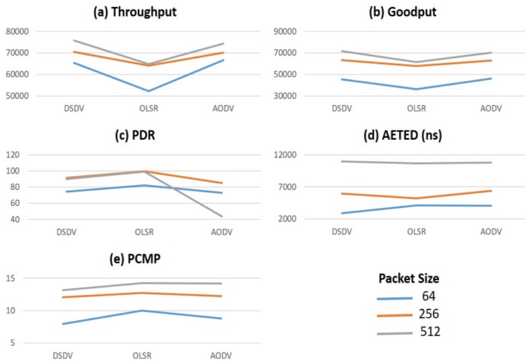
Fig. 5 NS3 simulation results with 30 nodes.
