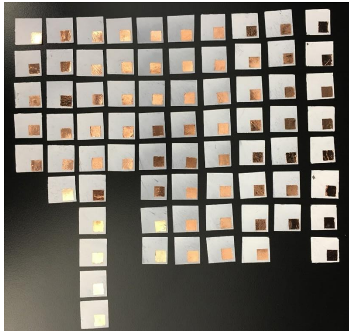
Figure 13. Some of the final fabricated and poled samples ready for testing.
